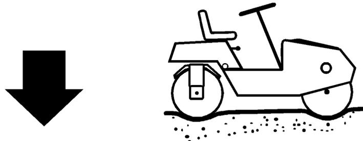
Vibrating Compactors (Figure 5-5): The motion of vibrating rollers or plates “shake” the soil particles into a more dense arrangement and works best with non-cohesive fills. Depending on the size and weight of the machine, vibrating compactors may be used close to the pipe. As always, care should be taken not to impact the pipe directly with a great deal of force.
