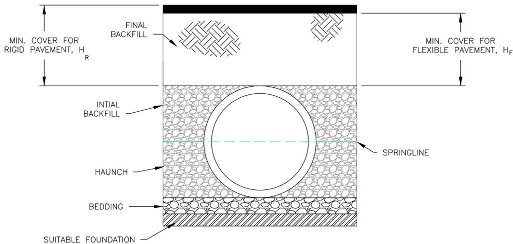
$H_R, H_F = 12"$  (0.15m) FOR PIPE DIAMETERS UP TO 48" (1200mm)
