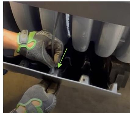
c. Continue to feed the zip tie through until the two halves of the coupler can be brought together and the zip tie can be cinched together.
