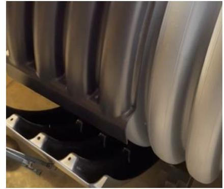
3. Notice that there are three holes located under the lip of each half of coupler. These are for the included zip ties to be threaded through and secure the coupler together. Make sure that the holes are aligned between the two halves of the coupler. If not, the coupler will not cinch easily and not create the needed soil tight fit.
