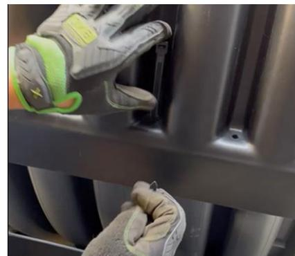
d. Complete securing the zip tie by feeding the pointed end of the tie into the square notch. Continue to pull the end of the zip tie through until a loose connection between the two lips of the coupler is created.
