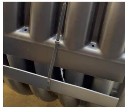
5. Repeat step four on the other side of the pipe, threading the zip tie through the outside of the coupler and continue working it through the hole on the inside of the part.
